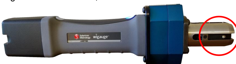
Application: DUSM with Multi Channel Wireless Handle for a Wireless Bore Gauge
