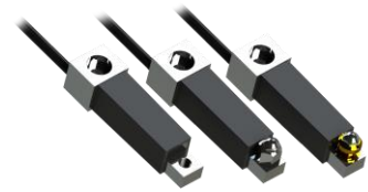
DUSM Mini Probe – Mini Single Leaf flexure with 0.5 mm range, IP 68 sealing, with multiple tip configurations
